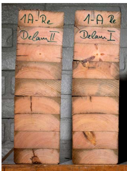
Figure 3.2 Delamination test pieces from beam 1A
