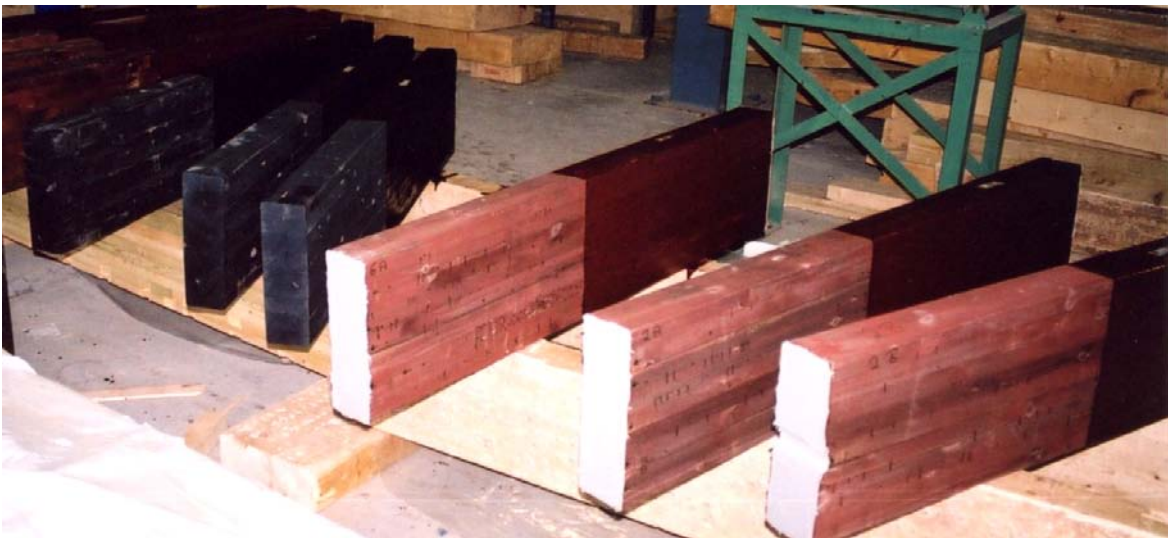
Figure 2.5 Surface treatment of the right beam sections with two different stains
