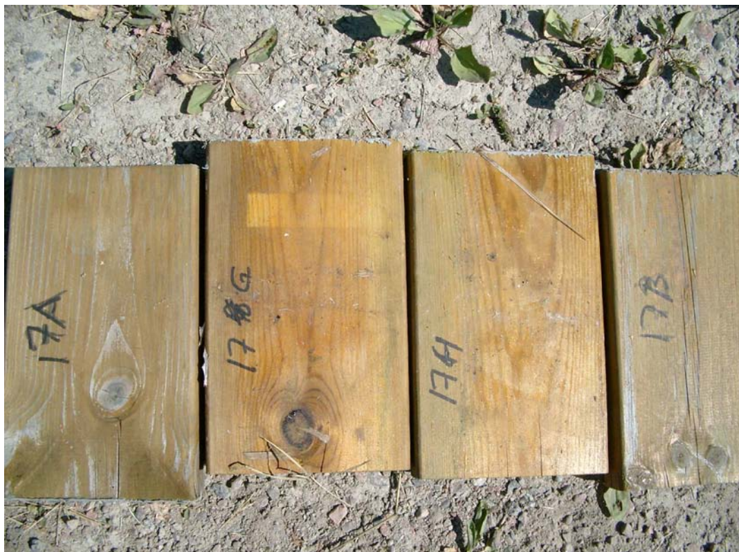
Figur 177. Furu, Tanalith E 7, pigmentert alkydolje.
