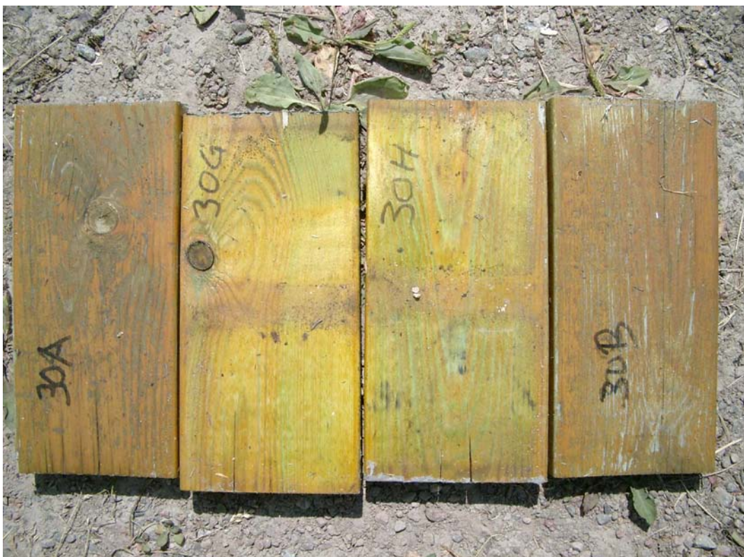
Figur 190. Furu, Tanalith M (farget), pigmentert alkydolje.
