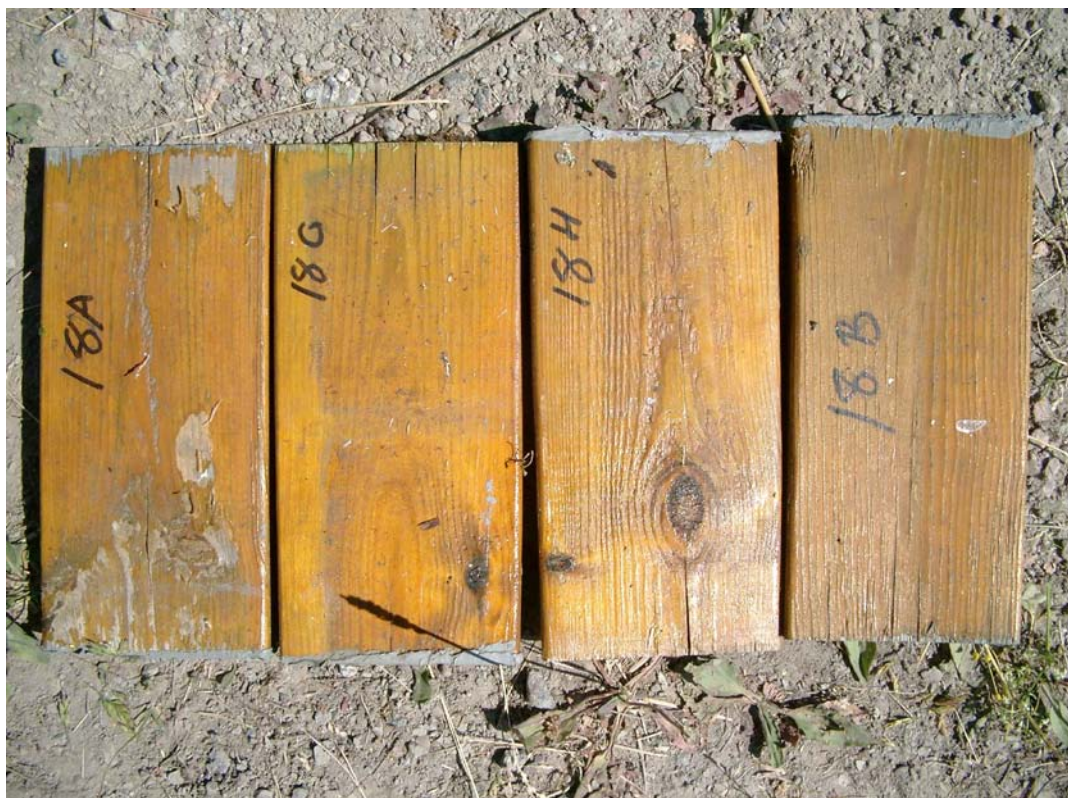
Figur 178. Furu, Wolmanith CX 8, pigmentert alkydolje.
