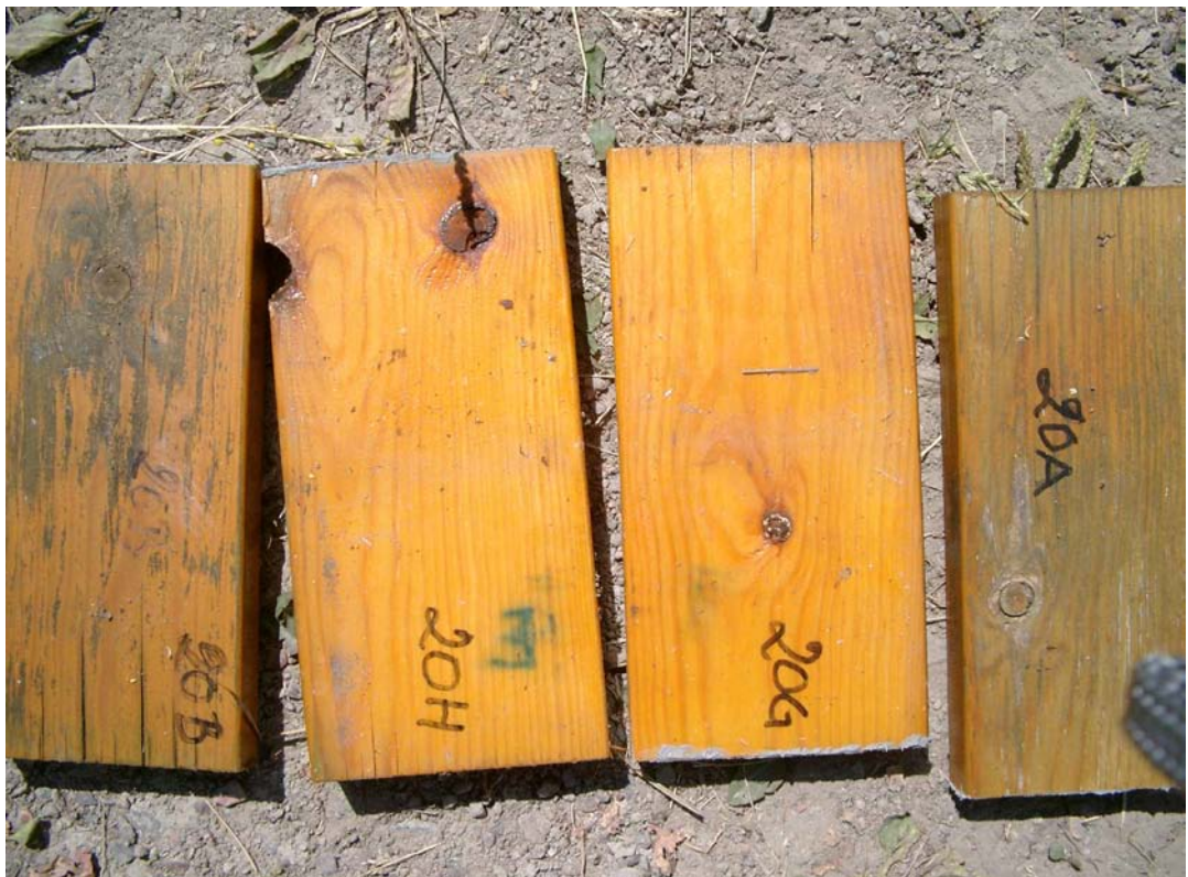
Figur 180. Furu, Scanimp, pigmentert alkydolje.
