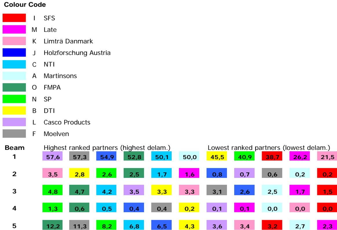
**Figure 5.6** Ranking for each partner and each beam, from the highest delamination (on the left side) to the lowest delamination (on the right side).
