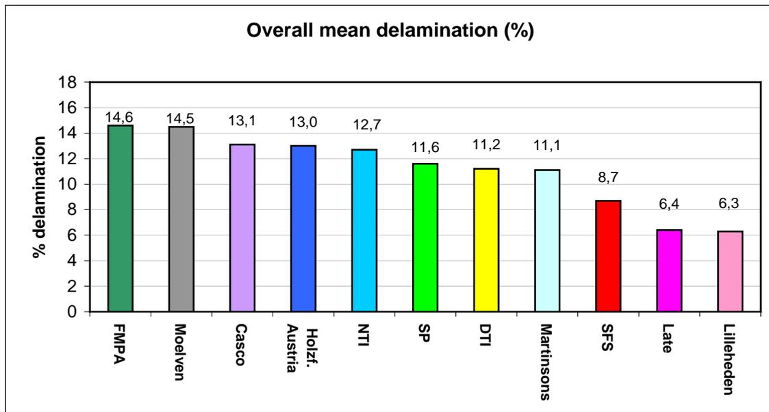
**Figure 5.7** Ranking for each partner and all beams, from the highest delamination (on the left side) to the lowest delamination (on the right side).
