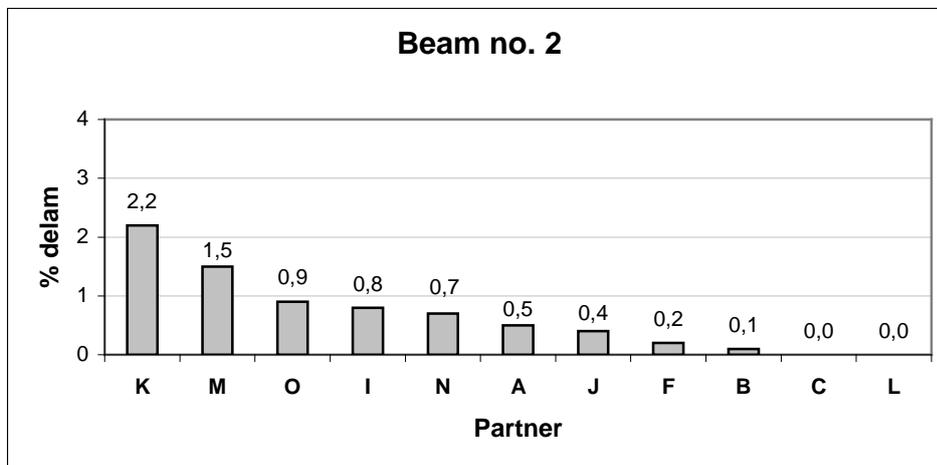
**Figure 7.2** Mean delamination for beam 2 (normal conditions)
