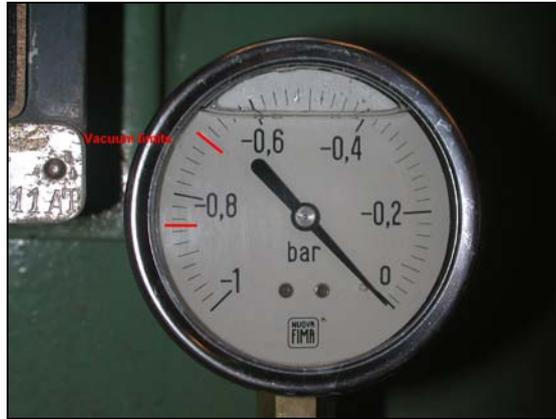
***Photo 1: With this meter, the vacuum to be drawn shall lie between -0,70 and -0,85 bar (0 is atmospheric pressure, -1 is absolute vacuum).***
