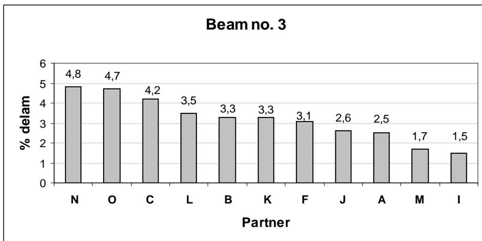
**Figure 5.3** Mean delamination for beam 3 (low glue spread)
