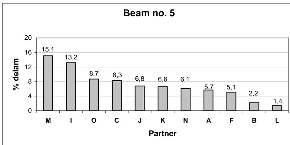
**Figure 7.5** Mean delamination for beam 5 (long assembly time, 55 min)
