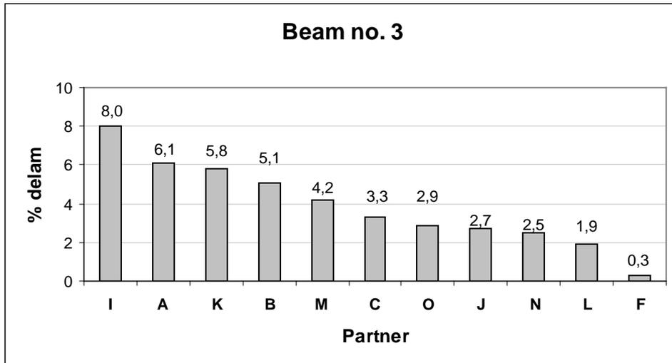
**Figure 7.3** Mean delamination for beam 3 (low glue spread)
