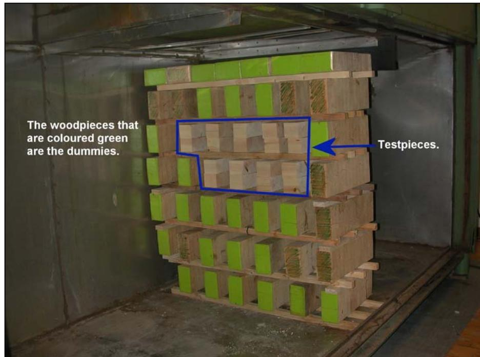
***Photo 2: Wet samples should be placed in the middle of the sample pile. Samples consisting of dry dummies and wet samples should fill out the whole of the drying chamber's cross-section. Samples shall always be placed above each other and stand in a row, so that a corridor of 5 cm between samples is present. The air speed shall be measured in the middle of the pile in between the samples, with a closed chamber door.***
