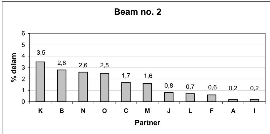
**Figure 5.2** Mean delamination for beam 2 (normal conditions)
