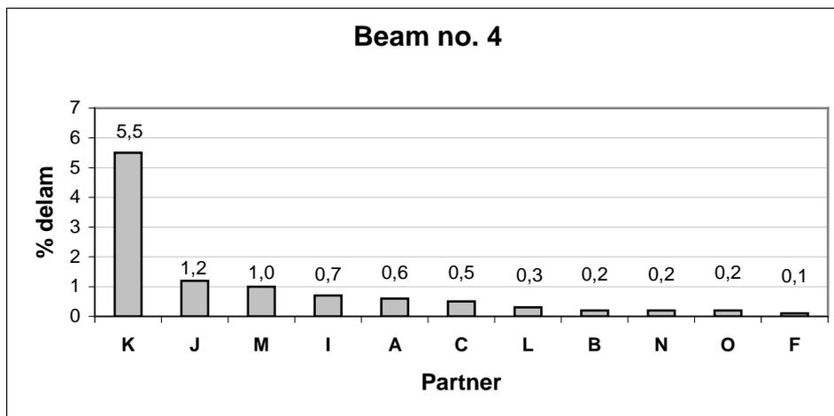
**Figure 7.4** Mean delamination for beam 4 (low pressure)
