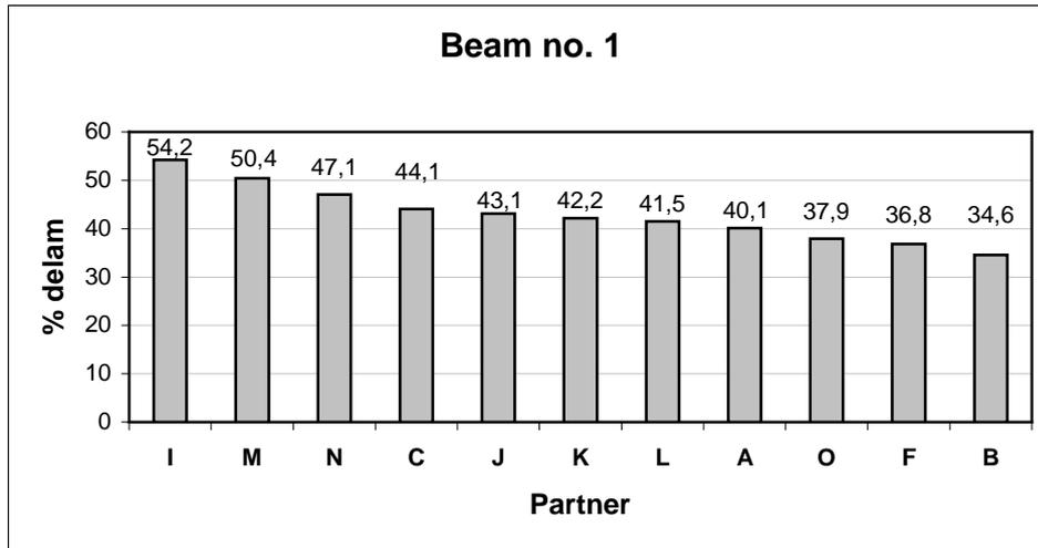
**Figure 7.1** Mean delamination for beam 1
