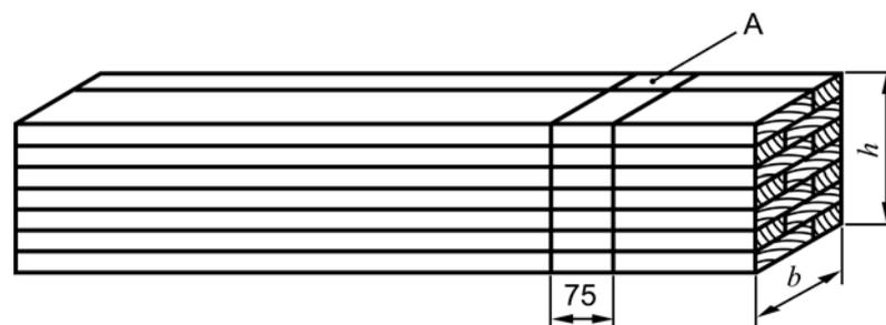
**Figure 1 - Test piece cut from a glulam member**
