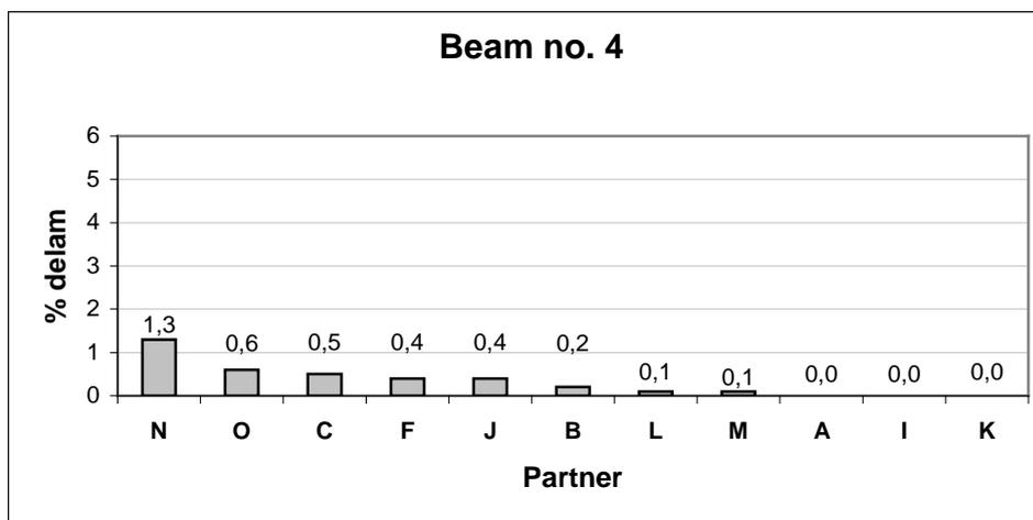
**Figure 5.4** Mean delamination for beam 4 (low pressure)
