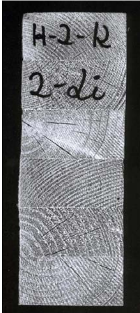
Figure 2.1. Part 1: Test piece EN 391-C.
